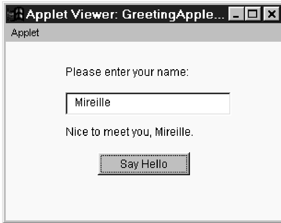
FIGURE 5.10 An applet viewer window running GreetingAppletWithButton after the user clicked on the button. This applet uses absolute positioning for laying out the GUI objects.
