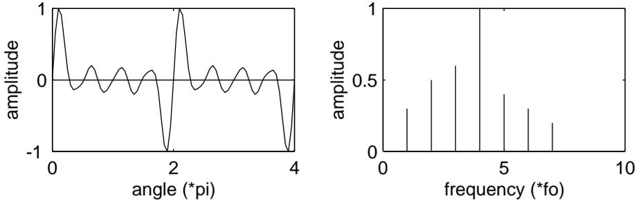
Figure 3: Waveform with higher power upper harmonics.
