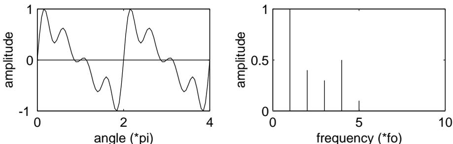
Figure 2: Waveform with lower power upper harmonics.
