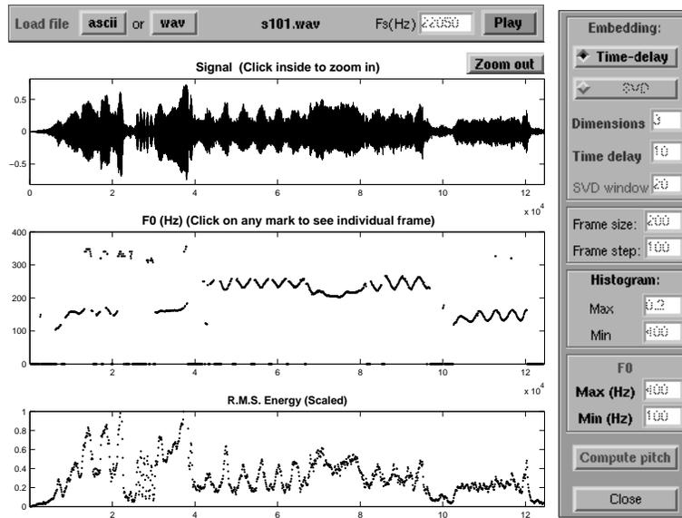
Figure 8: Terez's algorithm with subharmonic errors (singing).
